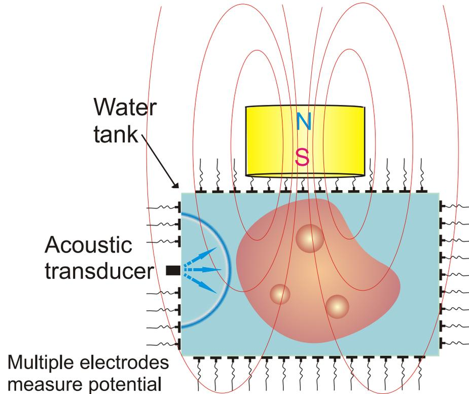
Separated charges create an electric field that's picked up by the electrodes
