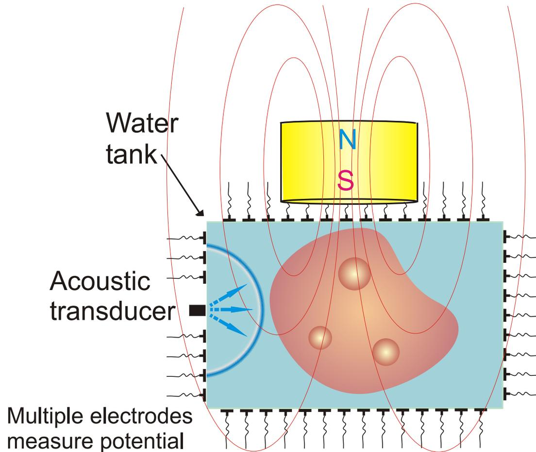
Ultrasound makes electrons and ions vibrate.
